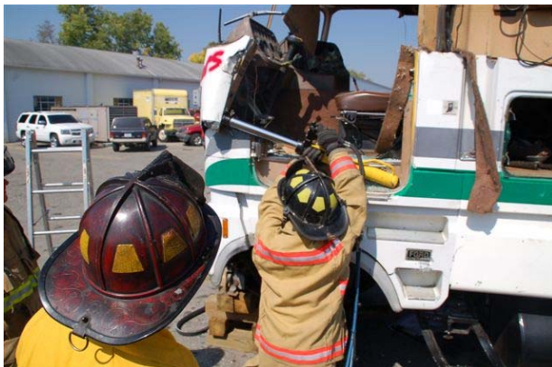
FFD Rescue Task Force personnel learning heavy truck dash displacement techniques using a Genesis 27/54 ram.
