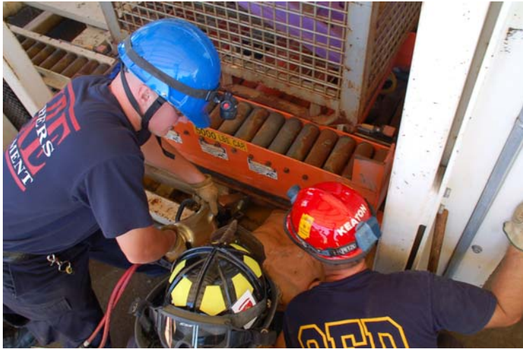
FFD Rescue Task Force personnel using a Genesis s50 spreader to complete a machinery rescue scenario for training.
