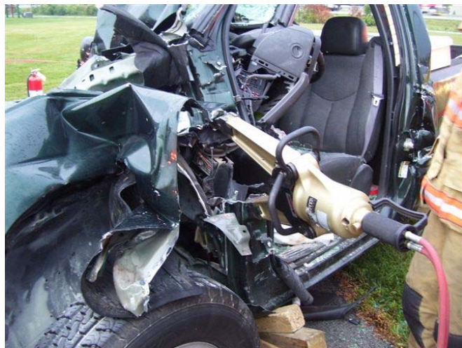
FFD personnel successfully extricated a middle aged man from this pickup by performing a dash lift with a Genesis s50 spreader.
